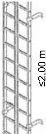
Fig. 5 Arrester rail mounted on the rungs of a fixed ladder or shaft ladder.
